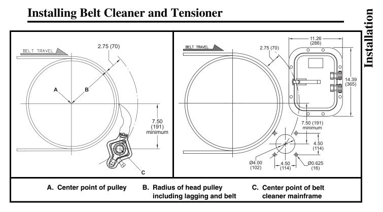
Figure 3. Belt Cleaner Mainframe Location & Chute Wall Cutouts for Martin<sup>®</sup> QB1<sup>TM</sup> Cleaner PV with Martin<sup>®</sup> Twist Tensioner
