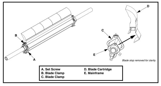
Figure 5. Removing and Installing Blade
