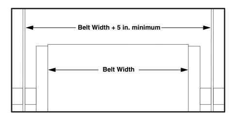
Figure 2. Chute Width Requirements
