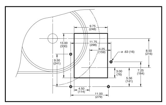
Figure 3. Operator Side Chute Cutout
