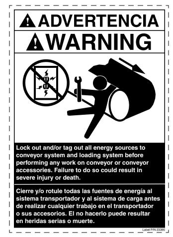
Figure 12. Martin<sup>®</sup> Conveyor Products Warning Label, P/N 23395
