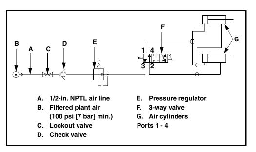
Figure 6. Air Cylinder Schematic
