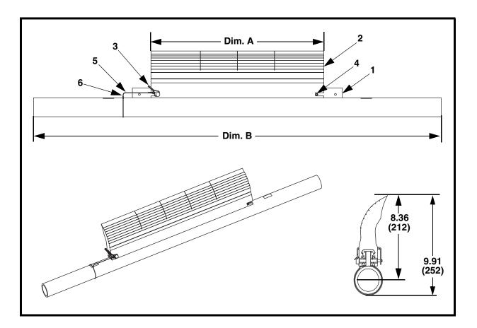
Figure 6. Martin<sup>®</sup> QC1<sup>TM</sup> Cleaner PD Assembly, P/N 38556-XXXXXXXXX
