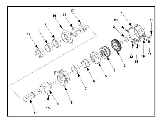
Figure 8. Martin<sup>®</sup> Twist Tensioner, P/N 38554
