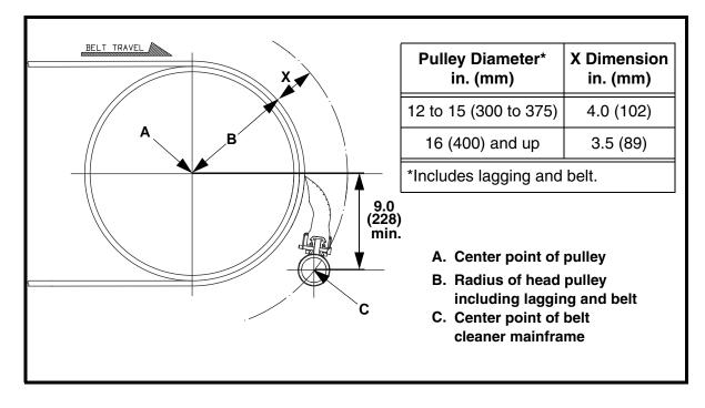
**Figure 1. Belt Cleaner Mainframe Location**
