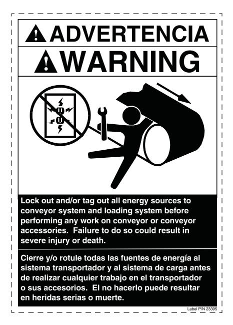
Figure 11. Conveyor Products Warning Label, P/N 23395
