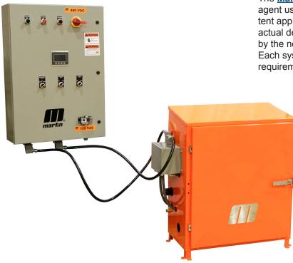
The <u>Martin<sup>®</sup> Surfactant Dust System</u> applies a surfactant agent using a fully automated system to maintain consistent application while avoiding surfactant agent waste. The actual details of the surfactant application are determined by the needs of the customer and the specific environment. Each system is custom engineered to match your operating requirements.
