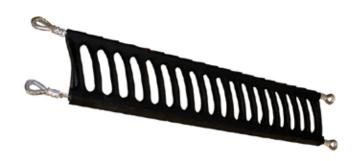
The <u>CleanScrape® Cleaner</u> is mounted diagonally on the discharge pulley and forms a three-dimensional curve. The cleaner has a matrix of tungsten carbide scrapers incorporated into the main rubber body during the vulcanization process. Despite a relatively low contact pressure between the belt and cleaner 85 to 95% of the adhering material is removed.
