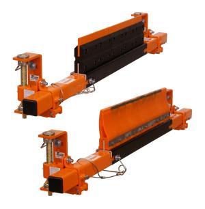
The Martin® SQC2S™ Cleaner incorporates individually-cushioned tungsten carbide blades for effective cleaning without risk to belt, splice, or blade. Installed in the secondary cleaner position, the Martin® SQC2S™ Cleaner's blade buffers cushion impact and maintains cleaning pressure.
