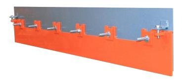
Installed outside conveyor transfer point skirtboards, EVO®\_External Wear Liner Retrofit Kit is an economical upgrade that improves skirtboard sealing and prevents spillage. Wearliner can typically be installed without requiring work inside chute or interfering with existing chute supports.
