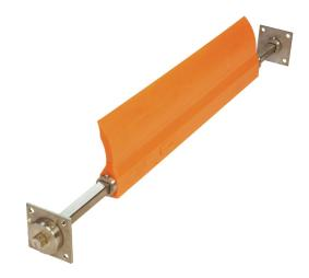
The Martin® Compact Cleaner from Martin Engineering uses a low-profile blade mounted on an internal square mainframe for effective belt cleaning in tight spaces. It is designed for applications on small pulleys and belts operating at speeds up to 350 fpm (1.8 m/sec).
