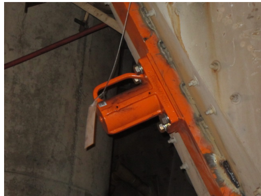
Cougar® Pnuematic Piston Vibrators are suited for use on any storage vessel.
