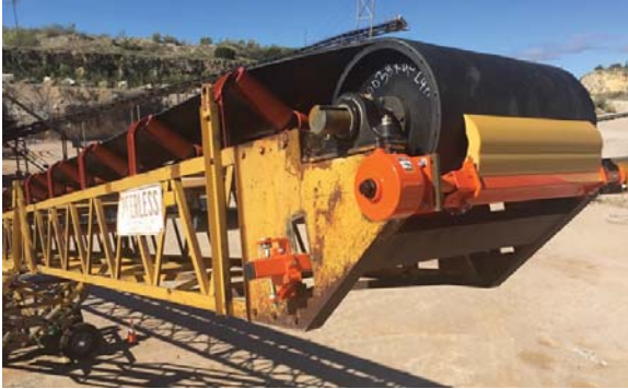
A Martin® QB1™ Cleaner HD was installed at the Hanson Burnette plant to address the excessive carryback.
