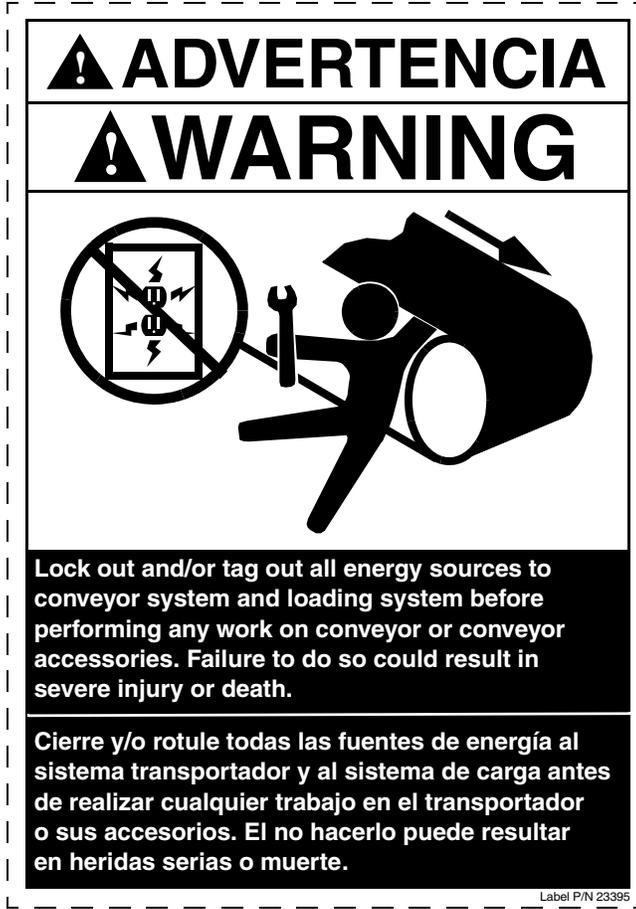
Figure 12. Martin® Conveyor Products Warning Label, P/N 23395
