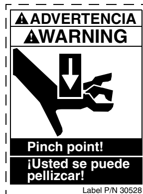
Figure 24. Pinch Point Warning Label, P/N 30528
