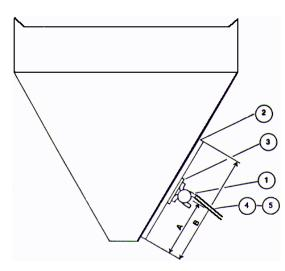
A = 1/3 of the length of the slope portion of the hopper.
