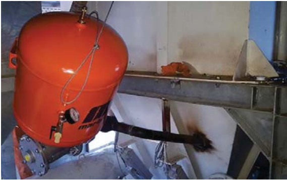
The tank and valve can be replaced easily without removing the pipe or nozzles.
