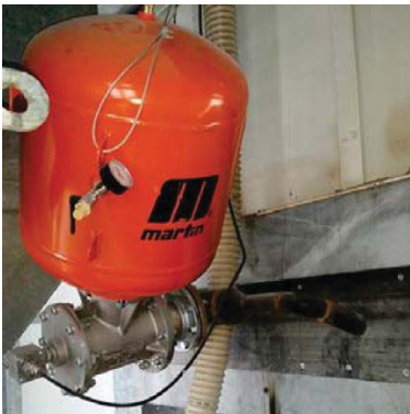
The split manifold creates a powerful discharge with a low impact on the central compressed air system.
