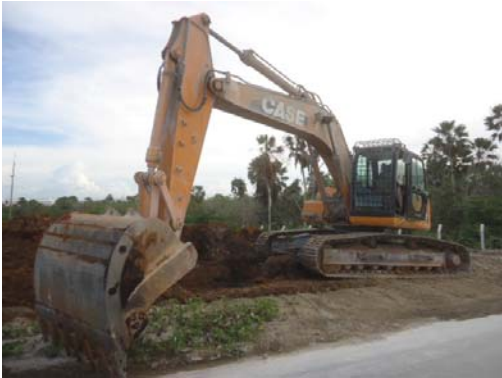
Cimento Apodi was experiencing wear damage to the underside of the bucket on its excavator.
