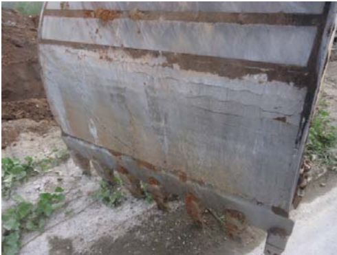
Martin® Arcoplate™ wear plate was installed across the face and around the curvature of the bucket.
