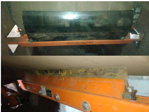
Hot material clung to the belt, requiring a high-heat blade to remove carryback and avoid premature wear.
