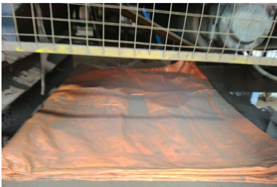
Hot material clung to the belt, requiring a high-heat blade to remove carryback and avoid premature wear.
