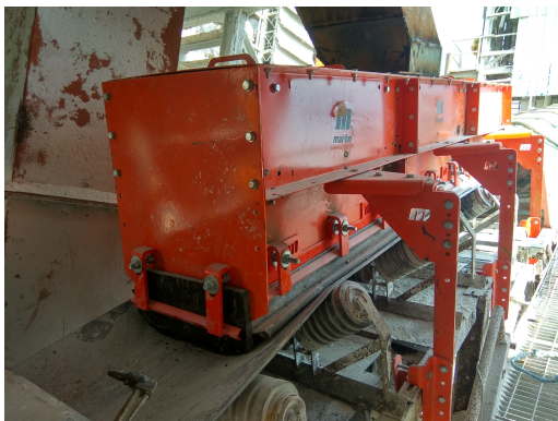
The modular chute box, sealing components & dust bags successfully contain the dry, powdered load.
