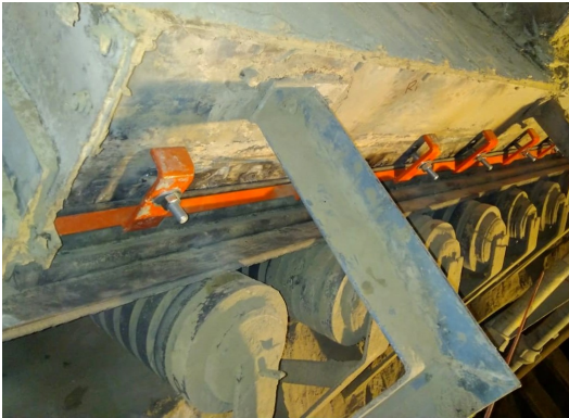
The team recommended and installed Martin® Apron Seal HD HR to withstand 120°C material temperature.
