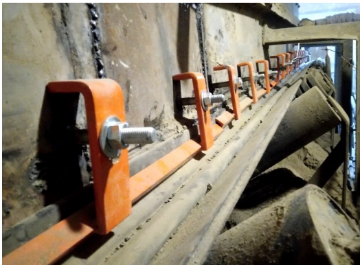
The installed solution significantly reduced dust and spillage, minimizing the manpower cost for cleanup.
