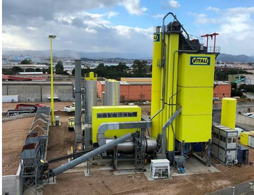
The Vitali Olbia facility handles ~2.19 million tons of sand & gravel per year to produce concrete and asphalt.
