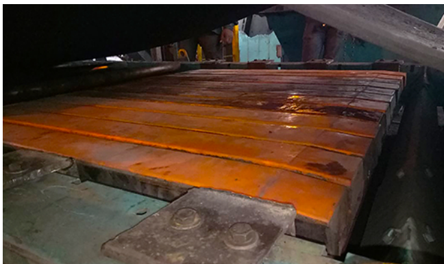
Placed under the transfer chute, the treated urethane bars offer impact protection with low friction on the belt.
