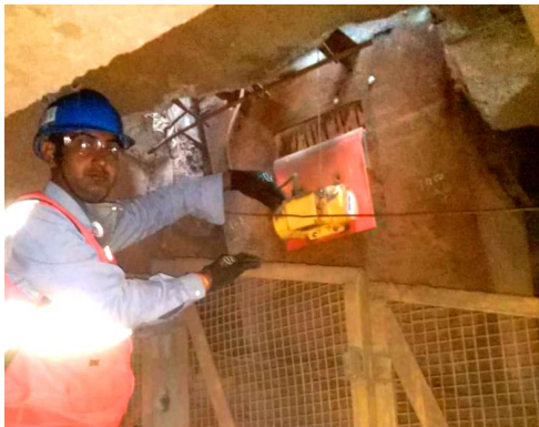
Vibrating Dribble Chute uses an electric vibrator and liner plate to avoid material clogging in discharge chute.
