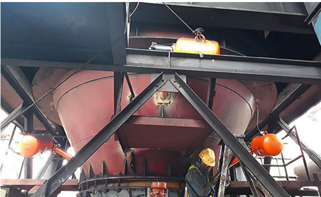
Located around the hopper at the discharge chute, the cannons dislodge accumulating cargo and aid flow.
