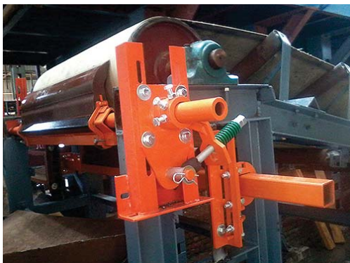
Spring tensioners ensure that the blade remains in firm contact with the belt, without damaging the splice.
