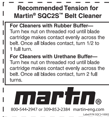
Figure 3. Martin® SQC2S™ Tensioning Label, P/N SQC2-10002
