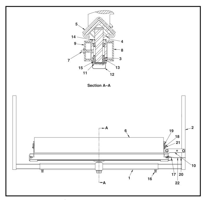
Figure 1. Martin $^{\circledR}$  Return Roller, P/N UCRR-007000-XXX\* (Sheet 1 of 2)
