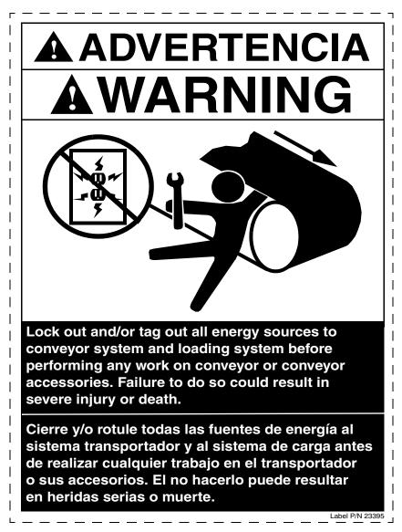
Figure 2. Conveyor Products Warning Label, P/N 23395
