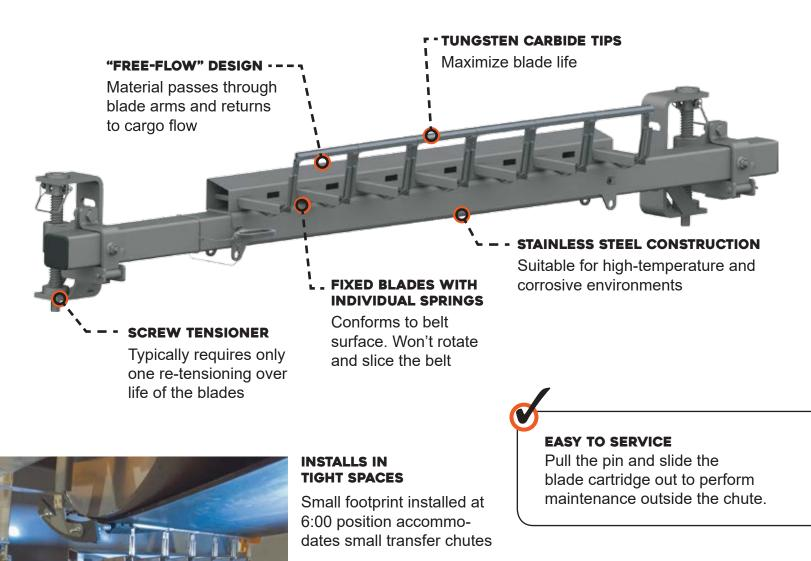
Keeps material in the material flow without the need for a dribble chute
