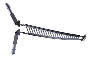
The <u>CleanScrape</u> <u>Cleaner</u> is mounted diagonally on the discharge pulley and forms a three-dimensional curve. The cleaner has a matrix of carbide scrapers incorporated into the main rubber body during the vulcanization process. Despite a relatively low contact pressure between the belt and cleaner 85 to 95% of the adhering material is removed.
