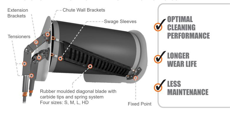
Installed diagonally at an angle across the discharge pulley forming a three dimensional curve, the revolutionary CleanScrape® Primary Cleaner requires minimal space for installation. The CleanScrape® Primary Cleaner incorporates a matrix of tungsten carbide tips and applies minimal pressure to the belt. Despite an extremely low contact pressure between belt and cleaner, 85% to 95% of stuck material is removed.
