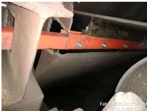
The DT2S features tungsten-tipped rubber blades to withstand medium-duty applications.
