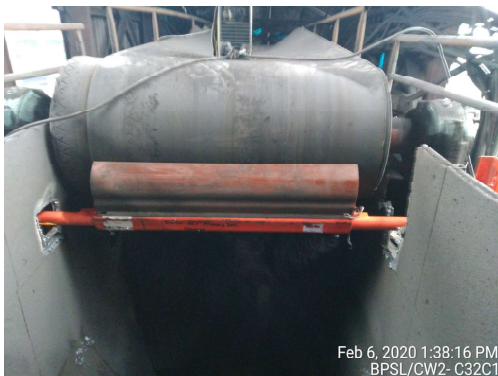
To replace the QB1 blade, one worker simply pulls the locking pin, unclamps the bracket and slides it out.
