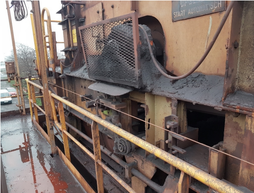
Fugitive material was causing lost cargo and forcing diversion of valuable manpower for cleanup.
