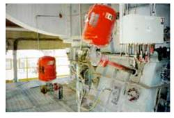
After the installation of the air cannons on the kiln, feed shelf, alkali bypass and riser duct, material flow through the pre-heater was more consistent.
