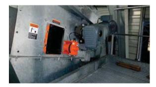
Martin installed belt cleaners and inspection doors which give access to the enclosure for maintenance and service.
