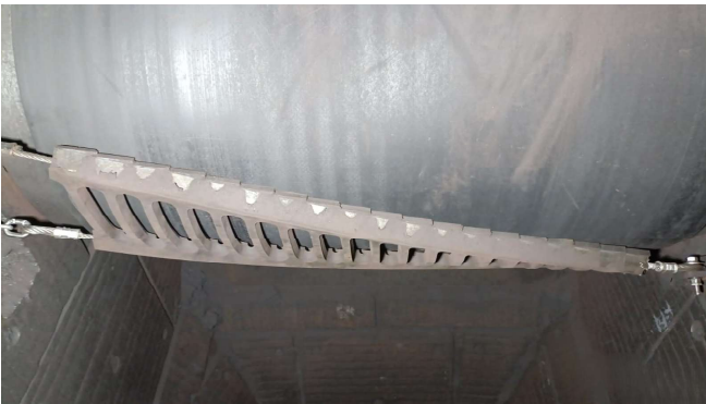
CleanScape® installed in minimal space, ensures optimal cleaning efficiency and longer service life
