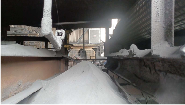
PU belt cleaners from other supplier were ineffective due to insufficient cleaning efficiency & rapid blade wear
