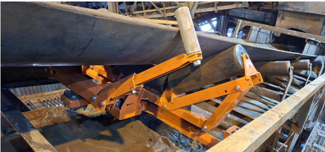
Martin® Tracker™ installed on the carrying side of 1200 mm wide conveyor belt
