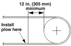
Figure 1 Installation position
