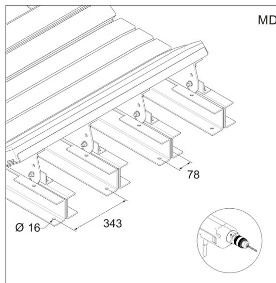
Notice: If the beams protrude sideways, they should be shortened and flush with the conveyor structure.
