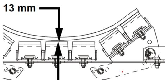
When installing one or more Impact Cradles, it is necessary to verify there is adequate power in the conveyor drive to compensate for the additional frictional drag.
