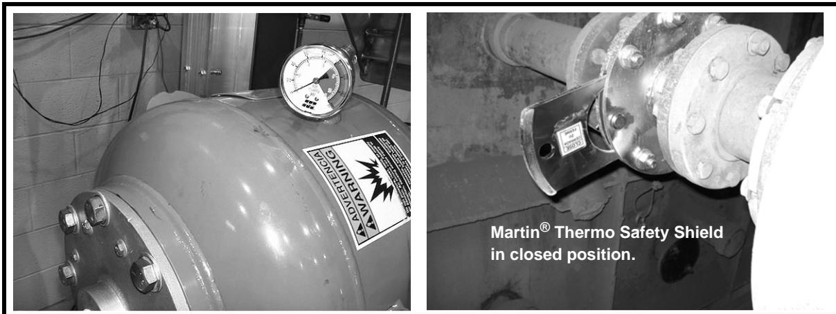
1. De-energize the air cannon; completely drain all compressed air energy from tank.
