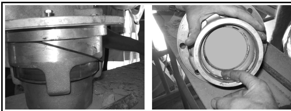
7. When replacing the valve assembly on the tank, a small amount of grease will secure the O-ring. Make sure O-ring stays secure during the reassembly.
