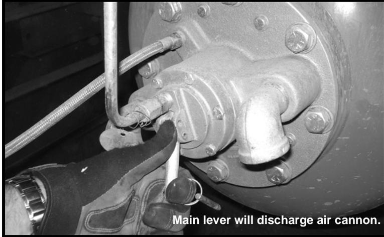
2. Close safety slide gate if equipped with one. If your air cannon has an open discharge port, make sure you are safely isolated from free-flowing material or hazards inside the discharge area.
