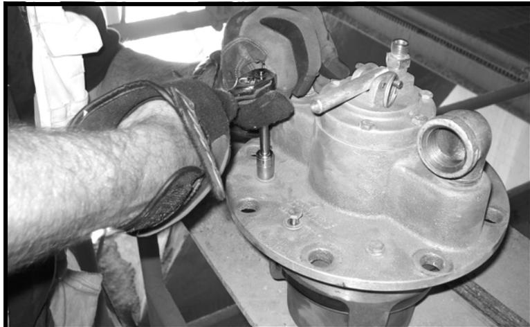
7. When replacing the valve assembly on the tank, a small amount of grease will secure the O-ring. Make sure O-ring stays secure during the reassembly.
