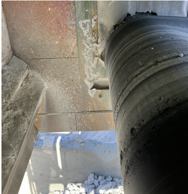
Persistent carryback accumulated along the return belt
