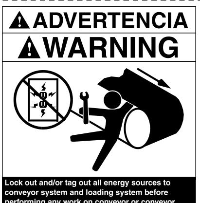
conveyor system and loading system before performing any work on conveyor or conveyor accessories. Failure to do so could result in severe injury or death.
