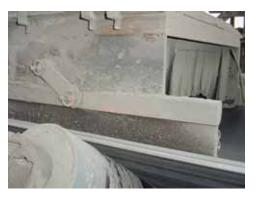
Mounted on pivoting pressure arms, Martin® Self Adjusting Skirting floats on the belt, and automatically self-adjusts to maintain effective sealing pressure.
