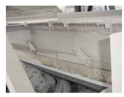
Installed on the clinker conveyor at Lehigh Cement, Martin® Self Adjusting Skirting has improved the effectiveness of the skirtboard seal while greatly extending the life of the sealing strip.
