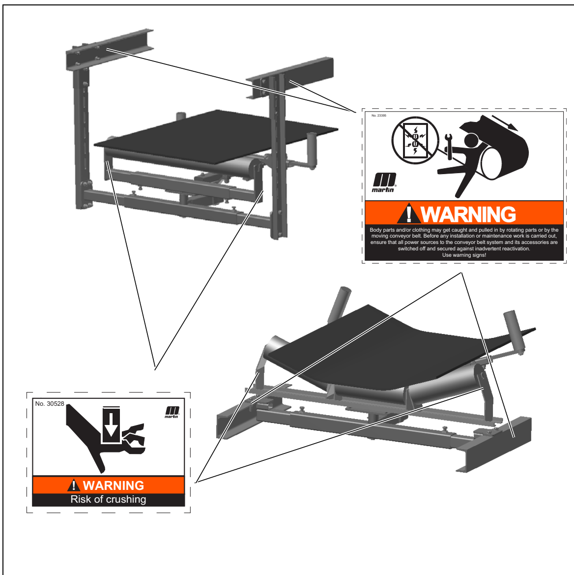
Fig. 27: Conveyor Products Warning Label
