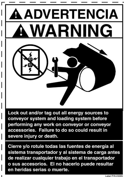
Figure 14. Conveyor Products Warning Label, P/N 23395
