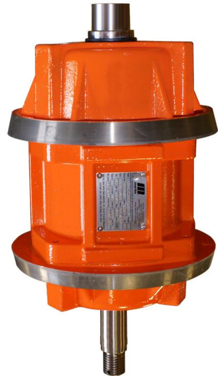
Martin Engineering MFS and MFD-Series vibrators are typically used in medium and large sieves and circular screens. They are rated at  $\frac{1}{3}$ ,  $\frac{1}{2}$ , and  $2\frac{1}{2}$  hp and are capable of producing forces up to 10,000 lbs.
