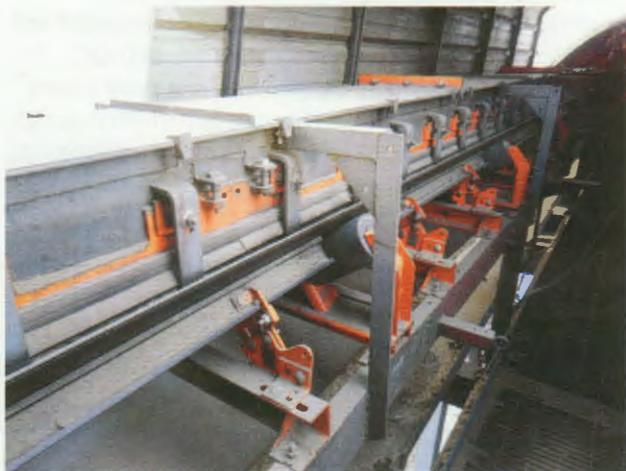
**Figure 3.** The project included upgraded transfer points to eliminate belt sag and improve sealing, as well as belt cleaning and alignment systems.
