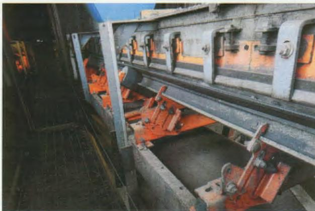
**Figure 4.** Technicians installed three impact cradles in the loading zones on each conveyor to create a flat edge for improved containment.
