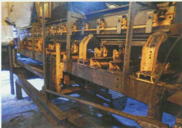
**Figure 2.** The twin belts have two load zones each, which were among the main points of concern.
