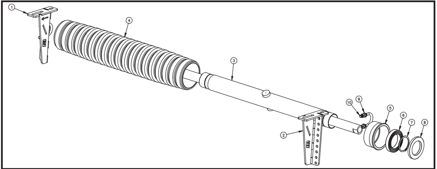
**Figure 4. Martin® Roller Tracker™ Assembly, P/N CTRSXX**
