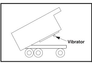
Figure 2. Locating Vibrator on Truck Bed
