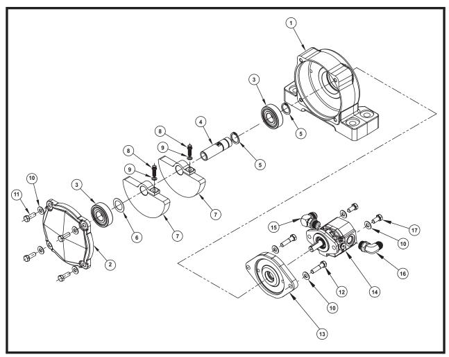
Figure 4. Cougar<sup>®</sup> THD Vibrator (Sheet 1 of 2)
