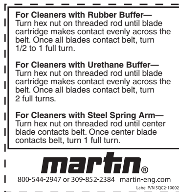
Figure 13. Martin ® SQC2S ™ Tensioning Label, P/N SQC2-10002
