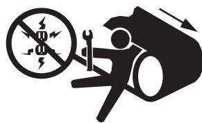
**Before installing, servicing, or adjusting the belt cleaner/tensioner, turn off and lock out/tag out all energy sources to the conveyor and conveyor accessories according to ANSI standards. Failure to do so could result in serious injury or death.**
