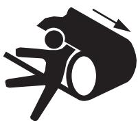
**Do not touch or go near conveyor belt or conveyor accessories when conveyor belt is running. Body or clothing can get caught and pull body into conveyor belt, causing severe injury or death.**
