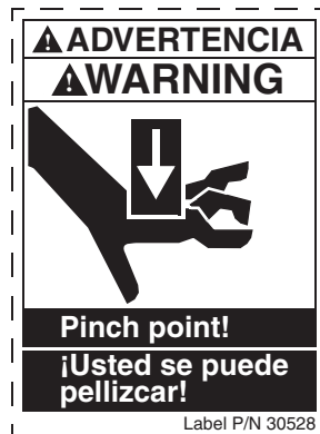
Figure 11. Pinch Point Warning Label, P/N 30528
